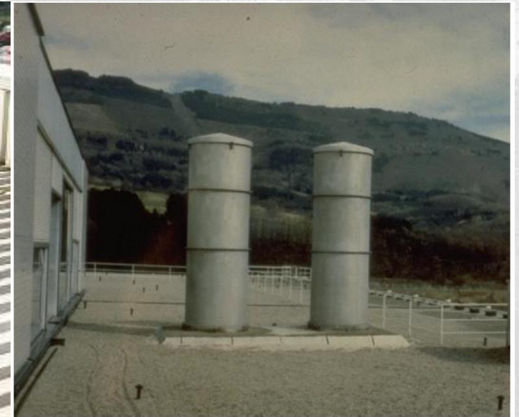
Figure 9-14. Tested metal covers held by rubber bands (the retaining wires for the covers are not visible)
